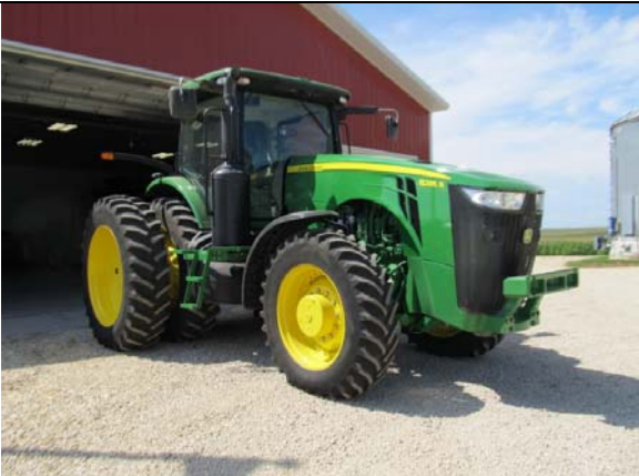
2014 John Deere 8285R MFWD tractor, 46" rear duals with inside weights; front weight bracket without weights, 34" front, buddy seat, 16F/5R Speed PowerShift, Independent Link Suspension with hydraulic differential lock, Deluxe Commandview II cab, quad hydraulics, 3 pt & Cat 4 adjustable swinging drawbar, front & rear fenders, cold weather starting kit, Power Tech PSC9.0L (549 cu in) 6 cyl IT4/Stage 3b compliant diesel, 7" color touch display, just 532 hrs, SN# 084947 - - 2 years remaining on PowerGard Protection Plan. There is a set of front weights that will sell separate (not part of original tractor purchase).
