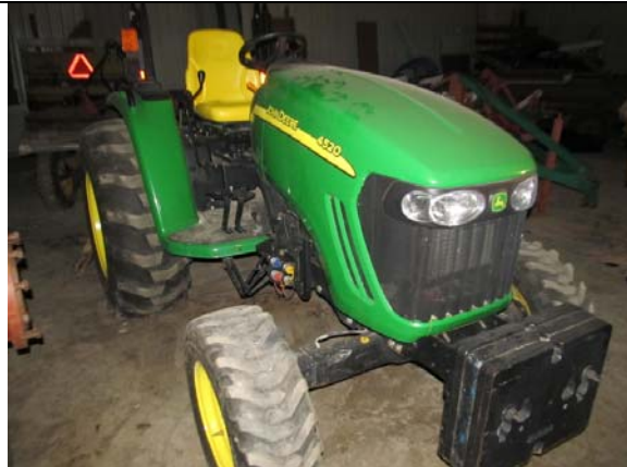
2010 John Deere 4520 PowrReverser MFWD compact utility tractor, open station with ROPS, 3 pt & standard, dual hydraulics, rear fenders, 17.5L rubber, front weights, only 92 hrs, SN# 755116
